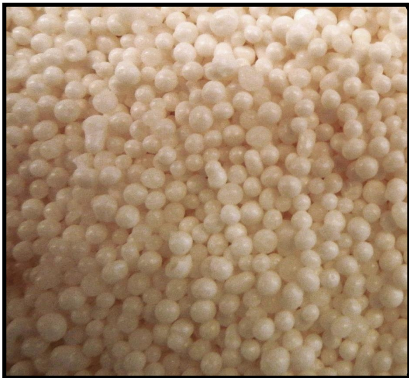
Prills (pellets) of FGAN piled in wooden storage bin
