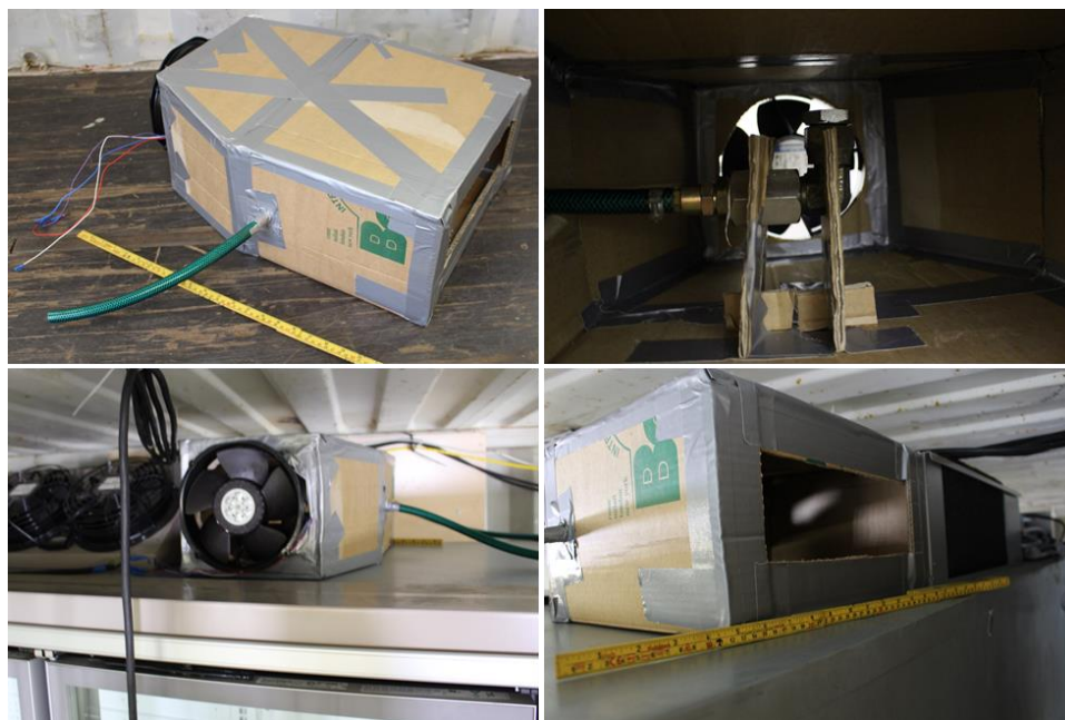
Figure 3.4: Mock-up condensing unit, variable-speed fan, and release orifice positioned to cause impingement against the roof of the housing.
