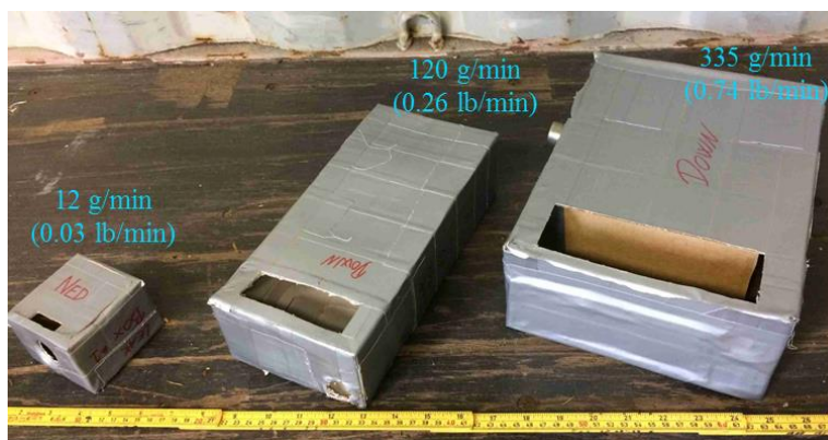
Figure 3.3: R-290 was released inside small boxes varying in size depending on the release mass flow rate to ensure release momentum was conservatively low.
