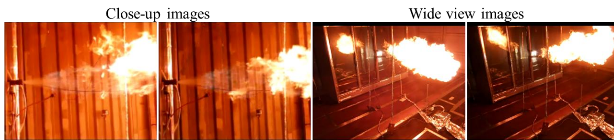
Figure 3.25: Jet flame of a liquid release through a 2 mm (0.08 in) diameter orifice.
